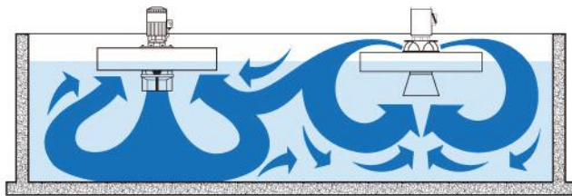
AquaDDM ® mixer with mechanical aeration.
