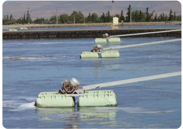
OxyStar® Aerators in Operation
