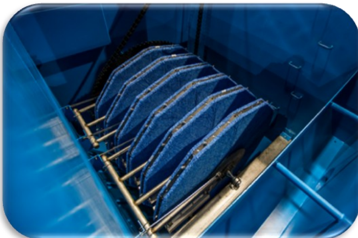
Internal components are assembled from 304 SS and non-corrosive materials for durability
