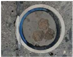
Cross-section of multi-tendon conduit
